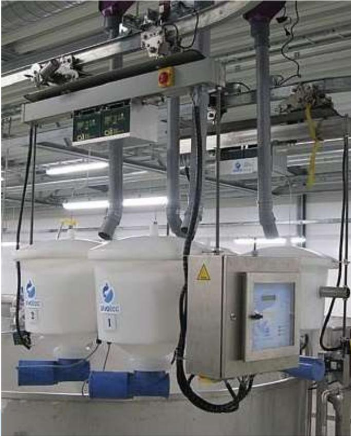
Arvo-Tec feeding robot improves feeding efficiency and saves labour time by feeding a large number of tanks with a single robot thus eliminating the need for a feeder at each tank.
