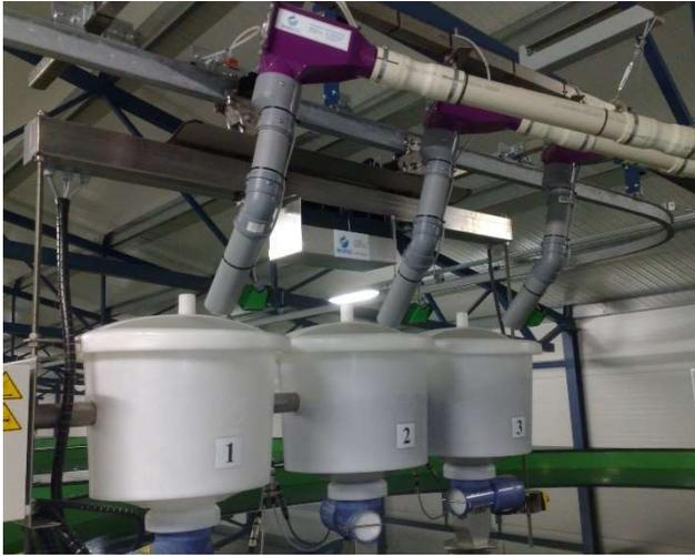
For the complete Arvo-Tec robot system; the automatic filling station adds further ease and efficiency to daily operations by managing the loading of the feed onto the robots.
