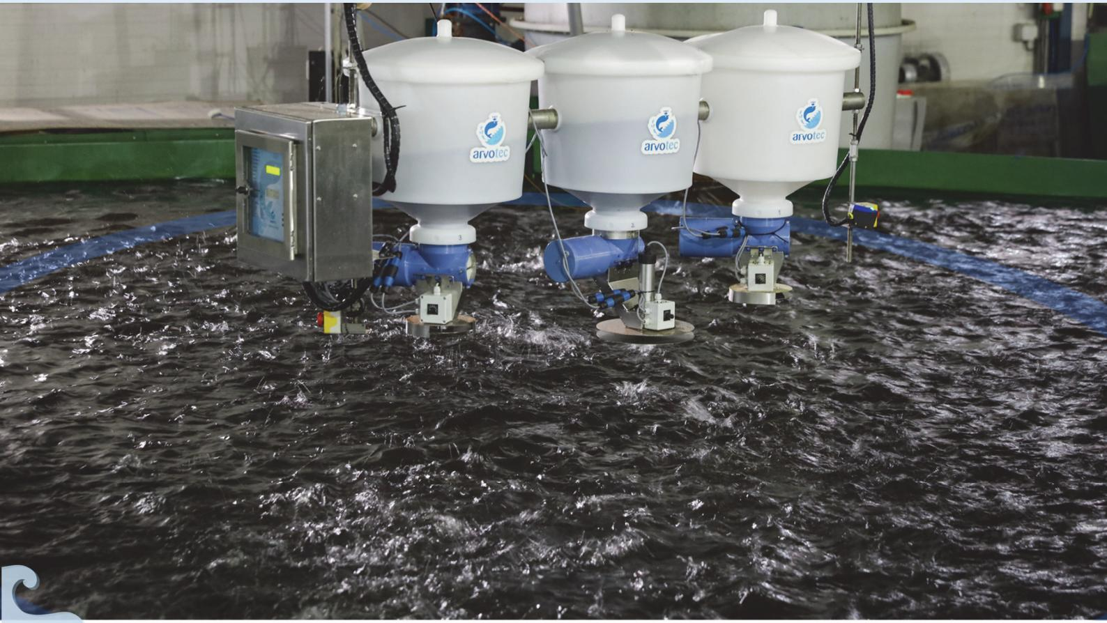
Arvo-Tec feeding robot improves feeding efficiency and saves labour time by feeding a large number of tanks with a single robot thus eliminating the need for a feeder at each tank
